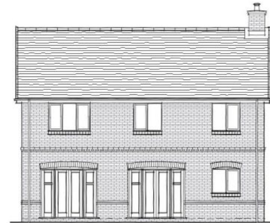
HEADERS, CILLS AND BRICK BANDING
