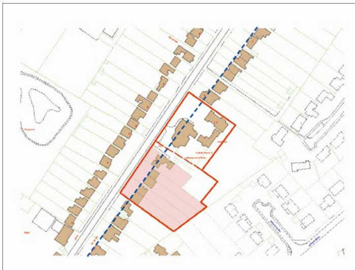
A location plan with the site hatched in red and the building line clearly indicated as a blue dotted line.
