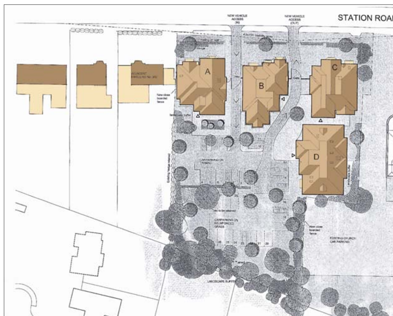
The plan for the proposed scheme. Note the large three-storey block to the rear of the plot overlooking the church and car-park, and the large communal parking area which fills most of the site not used by buildings.
